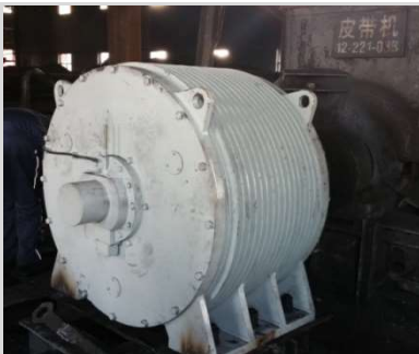
低速直驱 PM motor with Low speed and large torque
